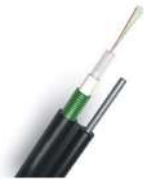
12 Core 2 FRP Cable, G652D Diameter 6.0, HDPE
