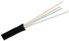
2 Core 2 FRP Cable, G652D Diameter 5.8, HDPE
