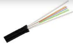
6 Core 2 FRP Cable, G652D Diameter 6.0, HDPE
