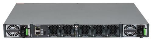
NSS5830-54XTQFP supports 48\*10G electric interfaces, 6\*100G QSFP28 optical interfaces, five modular fan slots, and dual modular power slots.
