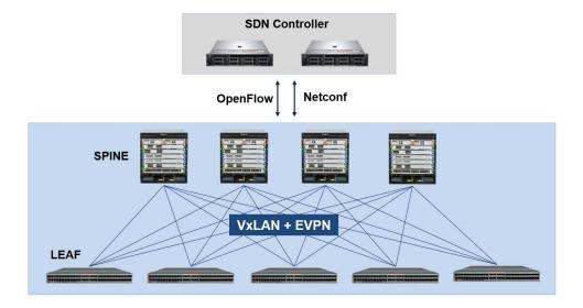
Fabric architecture has become a common and popular design option for building new-generation enterprise data center networks. Virtual Extensible LAN (VXLAN) and Ethernet VPN (EVPN) is essentially becoming the standard technology used for deploying network virtualization overlays in data center fabrics.
