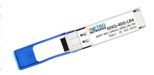
The central wavelengths of the 4 CWDM channels are 1271, 1291, 1311 and 1331 nm as members of the CWDM wavelength grid defined in ITU-T G.694.2. It contains a duplex LC connector for the optical interface and a 38-pin connector for the electrical interface. To minimize the optical dispersion in the long-haul system, single-mode fiber (SMF) has to be applied in this module.
